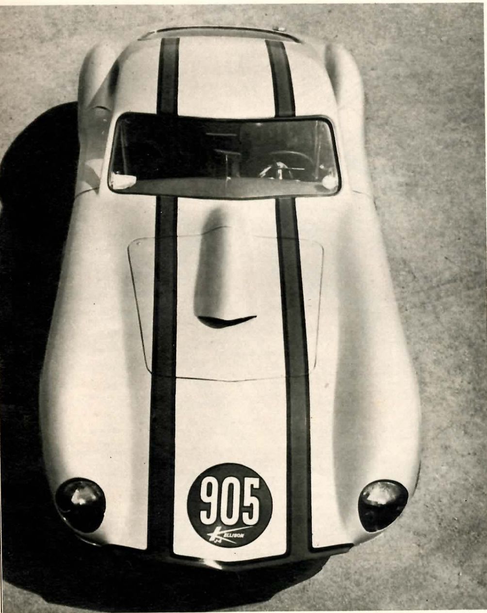
Projectile-like dimensions of the Kellison are readily apparent in this top view. The wind-cheating shape reflects the aircraft design studies of Jim Kellison.
