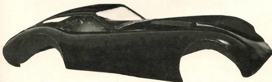
The J-4 Grand Turismo coupe drops onto a 98-inch wheelbase, and lists at $365 base, $605 as a complete body.
