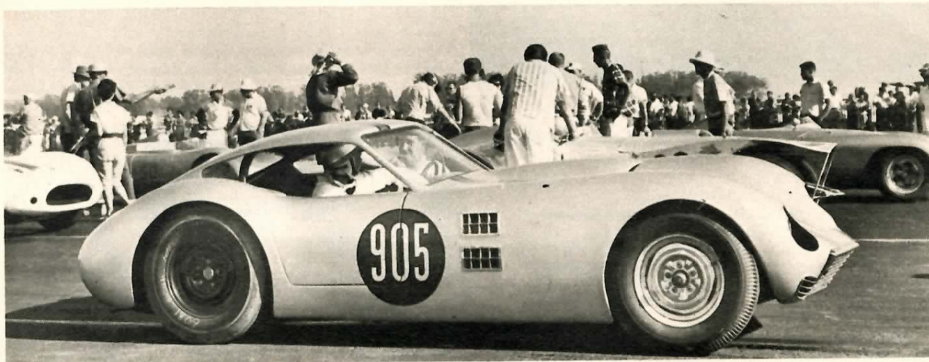
Low top features steel reinforcing bars through the pillars to the rear, provides excellent visibility through 360 degrees.
